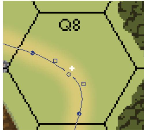
*Control Handles (square boxes) pulled away from their skeleton point (open circle) to make the road line follow the curve of the scanned road underneath.*
